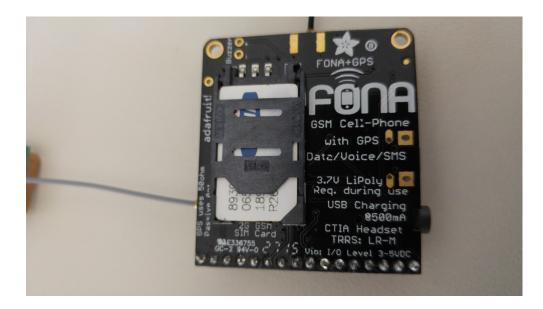
Figure 4.4. Back of the Adafruit Fona 808, the SIM slot is clearly visible
