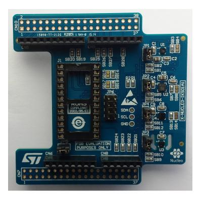
Figure 4.6. X-Nucleo IKS01A1 motion and environmental sensor shield
