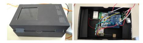
Figure 5.1. The cardboard case. On the right, the SwarmBike device inside the case
