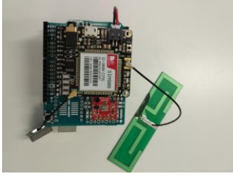
Figure 57: Assembly of the BMP180
