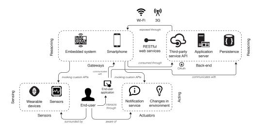
Figure 1: Proposed IoT systems reference architecture
